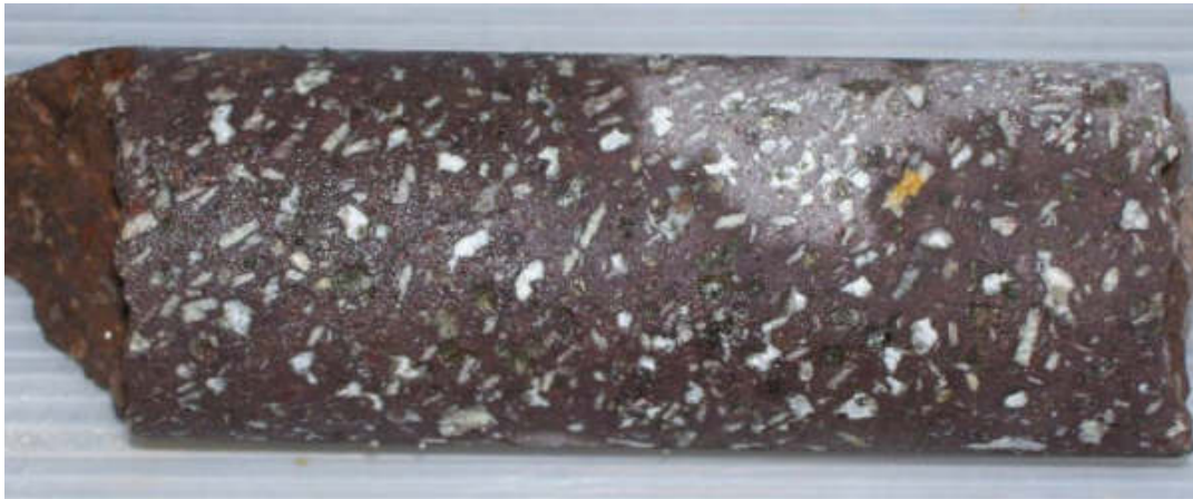
PHOTO 7: Basalt/Andesite Porphyry . It has a porphyritic texture with more than 20% plagioclase phenos and hematite in the groundmass. This rock type can be observed in the Magnolia Vein in drill holes DDH-07-M01 and M02.
