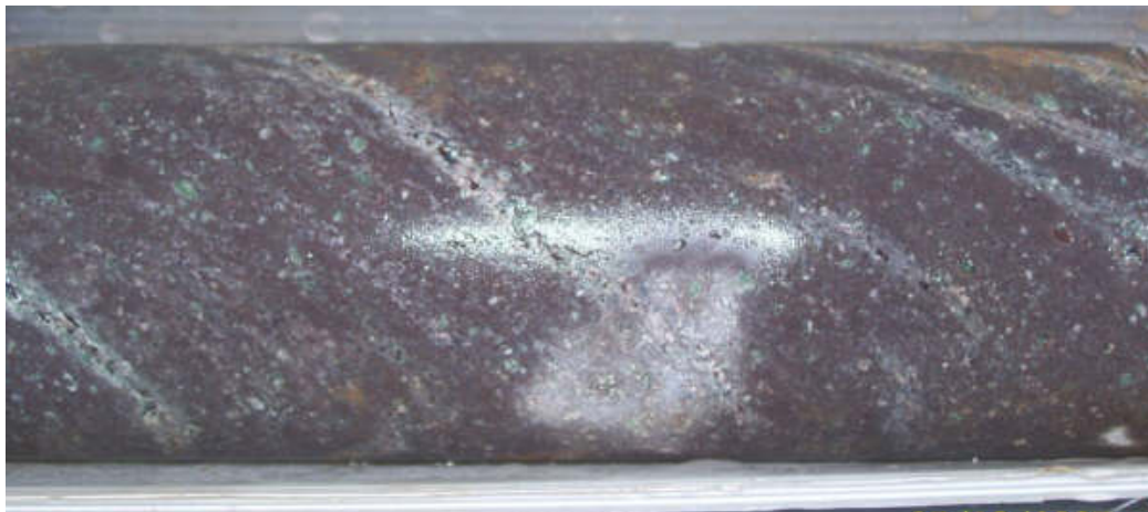
PHOTO 8: Basalt Porphyry : It has a porphyritic texture with 10% Plagioclase phenos, 3% chlorite and hematite in the groundmass. It exhibits a flow texture with orientation of the phenos. This rock type can be observed in the Esperanza Vein drill holes DDH-E01 and E02.
