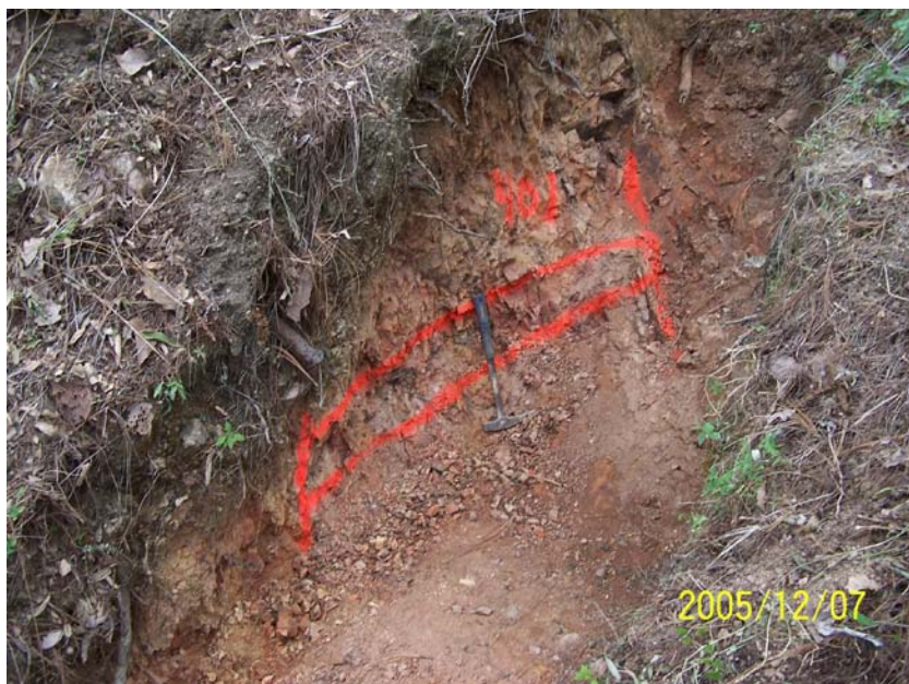
Plate 5: Quartz Vein in trench approximately 1 km NW of Florida-3 vein area. The vein width was 1.10 meters and returned 1.20 g/t gold and 123 g/t silver (Jaramillo, V., 2006)
