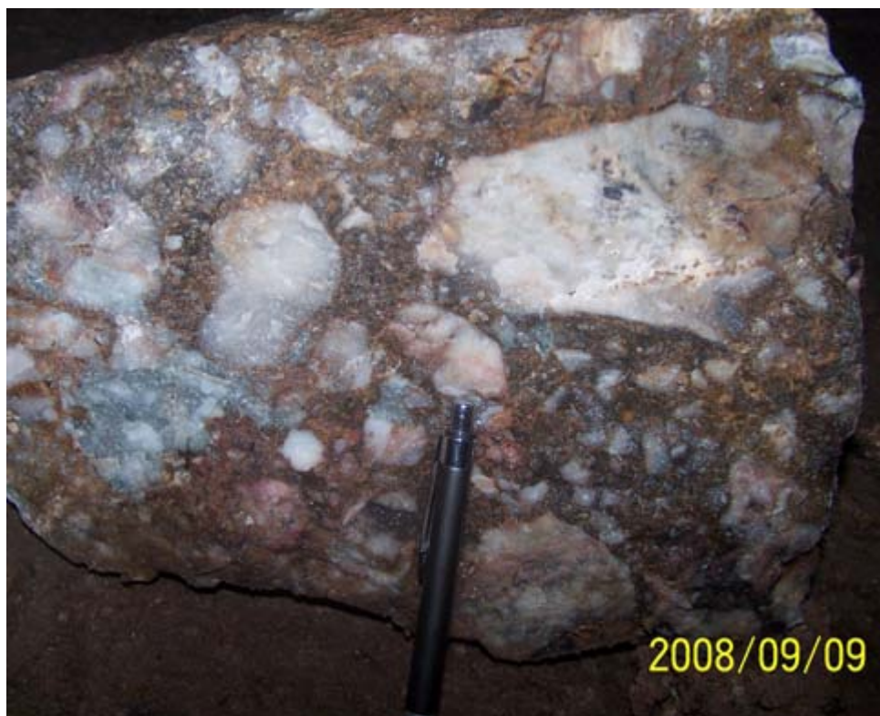
Plate 3: Hand specimen from Florida-4 Vein (level 1210m). It is a hydrothermal breccia which cuts through the main vein.
