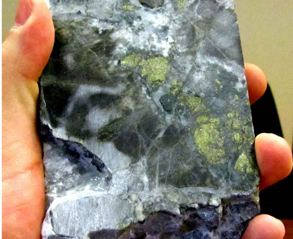
PLATE 10: Hydrothermal breccia with quartz-chalcopryite in matrix from CQ-107A (Sulfato South)
