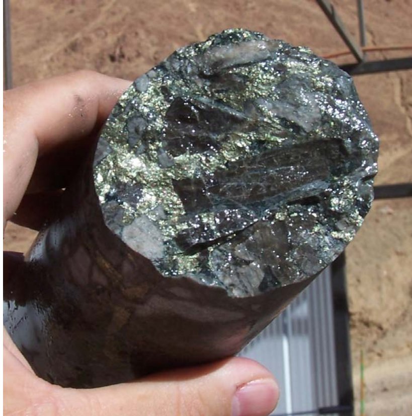
PLATE 6: Massive chalcopyrite in breccia matrix (CQ-100)
