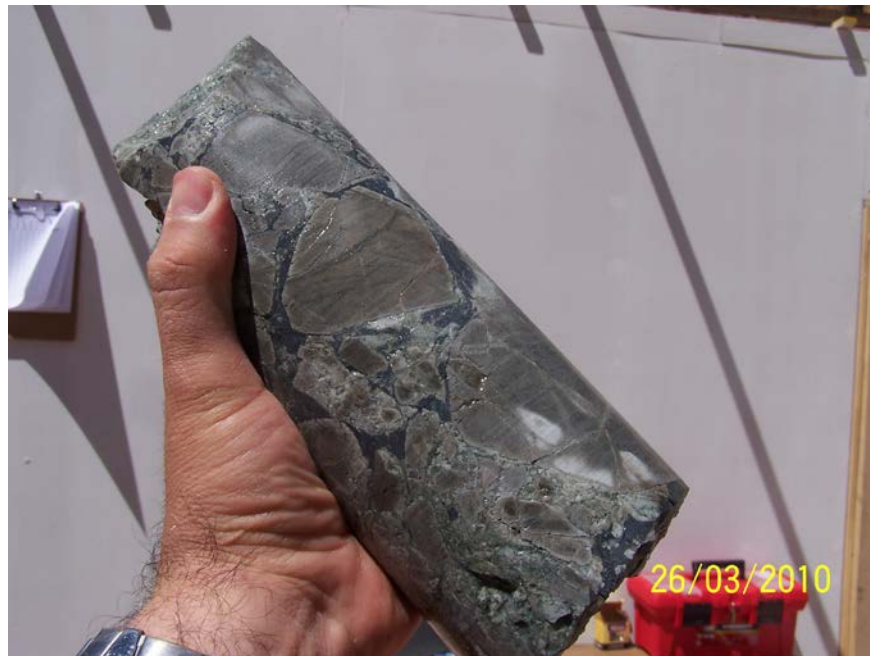
PLATE 7: Crackle breccia with massive chalcocite in matrix
