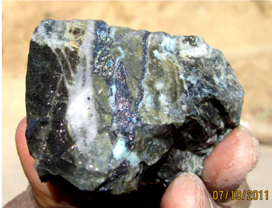
PLATE 8: Core fragment from Sulfato South with covellite
