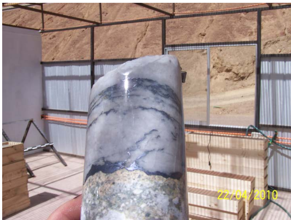
PLATE 11: Typical quartz-molybdenum vein in quartz monzonite porphyry at Cerro Moly
