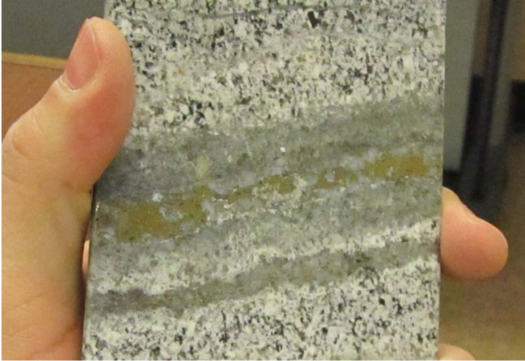
PLATE 12: Chalcopyrite-Quartz Vein in CQ-108 (Marta)
