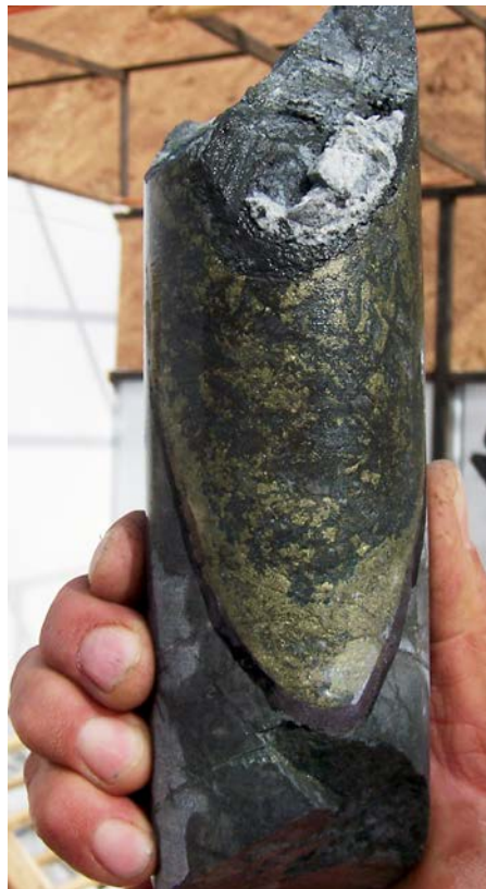
PLATE 9: Chalcopyrite-quartz vein from CQ-100 (Sulfato South)
