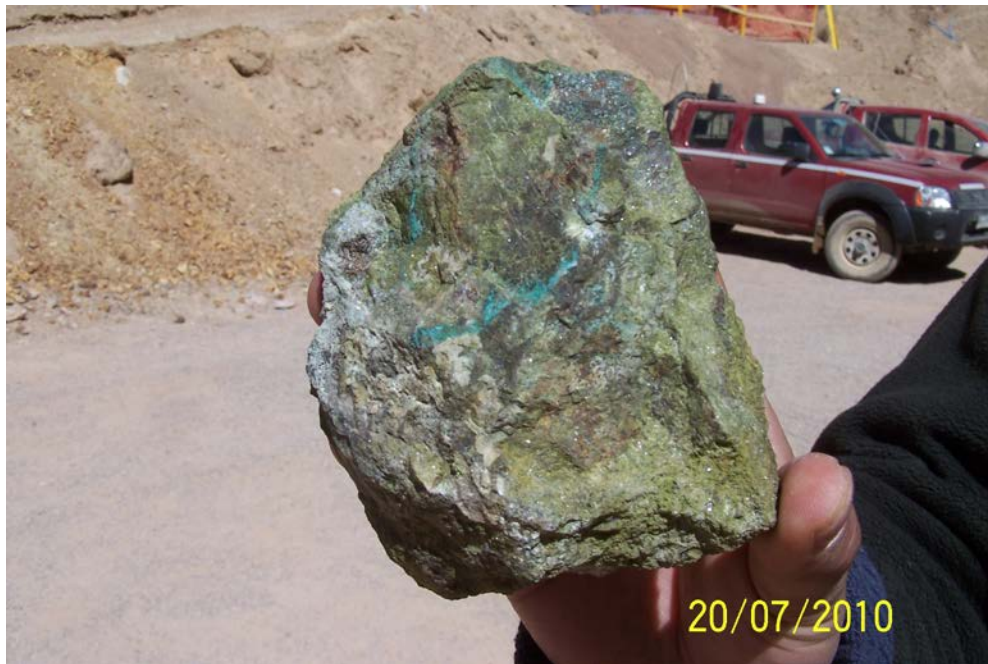
PLATE 15: Massive epidote fragment from Skarn zone, with clusters of Magnetite, impregnations of chrysocolla, veinlets of pyrite and blebs of chalcopyrite
