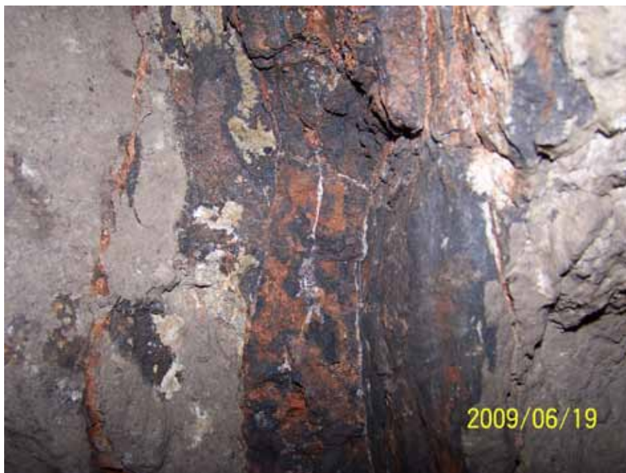
PLATE 4: Dark brown-black oxide vein 0.15m wide with < 1mm wide quartz veins within a mineralized fault structure 1.0m wide. Above Station 37.
