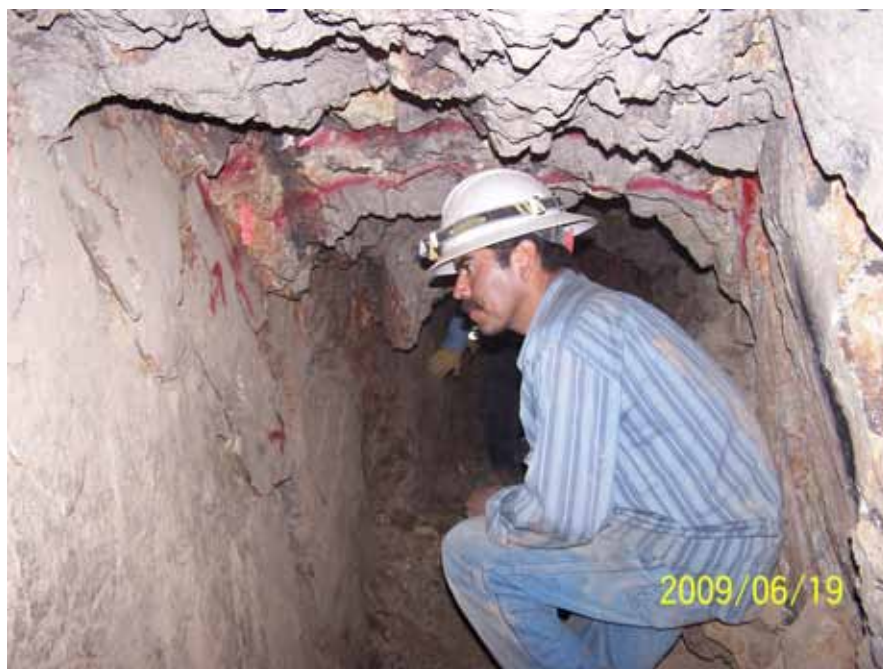
PLATE 5: Mineralized structure (fault zone) 1.0m wide. It contains several parallel veins as that shown in the previous plate. Sample No. 810534.
